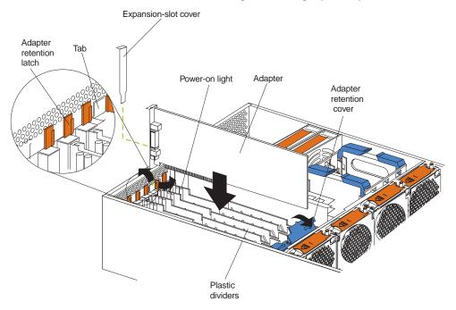
To install a hot-plug PCI adapter:
